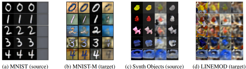
Figure 2: Reconstructions for the representations of the two domains for “MNIST to MNIST-M” and for “Synth Objects to LINEMOD”. In each block from left to right: the original image \mathbf{x}_t ; reconstructed image D(E_c(\mathbf{x}^t) + E_p(\mathbf{x}^t)) ; shared only reconstruction D(E_c(\mathbf{x}^t)) ; private only reconstruction D(E_p(\mathbf{x}^t)) .
