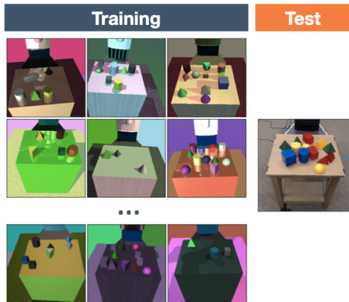
Fig. 1. Illustration of our approach. An object detector is trained on hundreds of thousands of low-fidelity rendered images with random camera positions, lighting conditions, object positions, and non-realistic textures. At test time, the same detector is used in the real world with no additional training.
